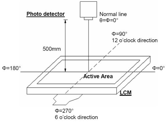
Figure 4.2 Optical measurement system setup
